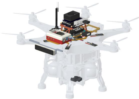
Control and communication subsystem
